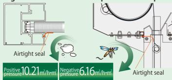
Further improved air-tightness in combination with an air tight seal. Possible to prevent the fully \*our product attach airtight seal; shown by numerically closed of insects and dust intrusion, and achieve a higher quality control and clean working environment
